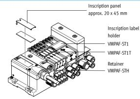
An inscription label holder VMPAF-ST1 (Part No. 546 228, code T in the order code, for holding paper labels) or VMPAF-ST1T (Part No. 544 422, for holding IBS-9x20 inscription labels) can be mounted on each manifold rail for labelling the valves.
