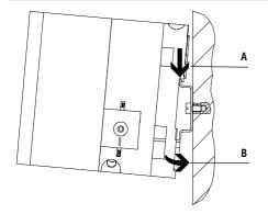
The MPA-F valve terminal is attached to the H-rail (see arrow A). The valve terminal MPA-F is then swivelled onto the H-rail and secured in place with the clamping components (see arrow B). For H-rail mounting of the valve terminal you will need the following MPA-F mounting kit:
