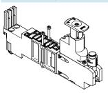
An adjustable pressure regulator can be installed between the sub-base and the valve in order to control the force of the triggered actuator. This pressure regulator maintains an essentially constant output pressure (secondary side) independent of pressure fluctuations (primary side) and air consumption.
