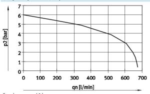
Supply pressure 10 bar, set regulator pressure 6 bar
