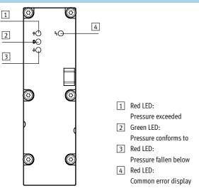
The pressure sensor indicates whether the applied pressure exceeds, conforms to or falls below the setpoint value using three LEDs. An additional LED indicates common errors (limit exceeded or fallen below). The limits for pressure monitoring are set by means of parameter settings. You can parameterise the pressure sensor plate via the PLC or the handheld device (CPX-MMI-1) from Festo.
