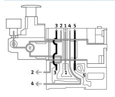
This pressure regulator regulates the pressure in duct 2 after the pressure medium flows through the valve. During venting, the exhaust flow in the valve is from duct 2 to duct 3 via the pressure regulator.
