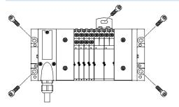
The MPA-F valve terminal is screwed onto the mounting surface using four M6 screws. The mounting holes are on the pneumatic interface and on the right-hand end plate. Optional mounting brackets are also available.
